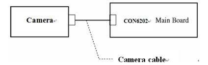
If a connector is disconnected, connect it firmly and repeat Procedure 1. If the camera is still not functioning properly, perform Check 2.
